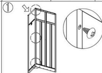
1 Bolt the left side and back plate with self-tapping screws (5x10).
