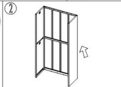
2 Bolt the right side with back plate in the same way as the first step.
