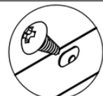
Bolt the left side and back plate with self-tapping screws(5x10)
